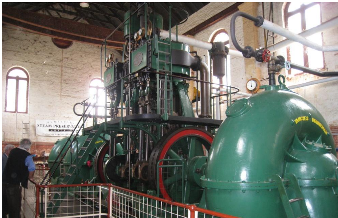
Psyche Bend triple-expansion engine flanked by two coaxial, centrifugal pumps either side
