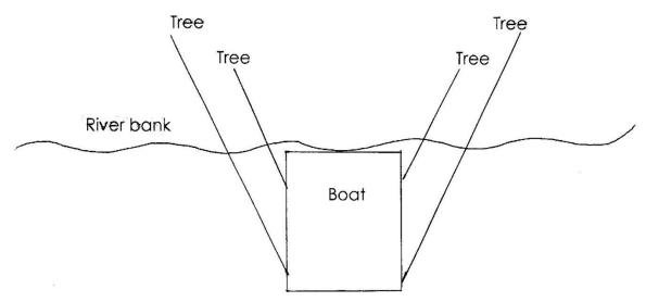
then the other back rope followed by the two front ones. Once *all four* ropes are secure, (winds can change dramatically overnight) place in neutral gear and turn the motors off. The skipper should always check the knots. A reliable knot for securing the ropes to trees or poles is the 'round turn & two half hitches'.
